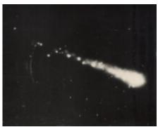
The trace of a single alpha particle obtained by nuclear physicist Wolfhart Willimczik with his spark chamber specially made for alpha particle.
